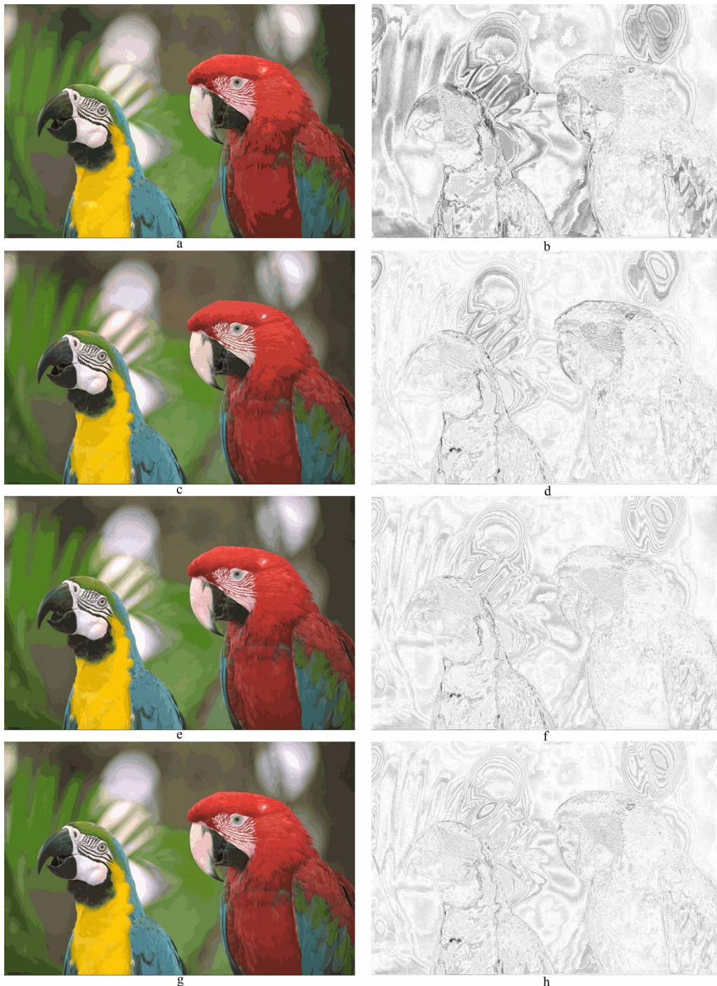
Fig. 3. (Color online) Sample quantization results for the Parrots image ( K=64 ): a, MC output; b, MC error; c, FKM output; d, FKM error; e, WSM output; f, WSM error; g, WSM-C output; h, WSM-C error.
